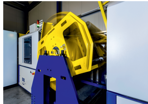
*ITT double inline setup for high bead to bead test capacity utilizing tread and belt package inspection from inside and both sidewalls from outside
